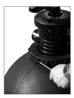
driver, loosen bolt on splitnut on valve a couple of turns.
