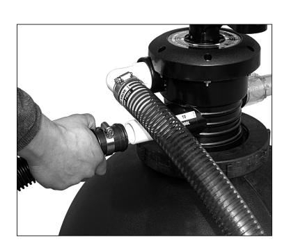
15. Install hose onto smooth hose adapter in valve by loosening hose clamp and sliding over adapter end. Install other end onto return fitting of pool and tighten clamps.
