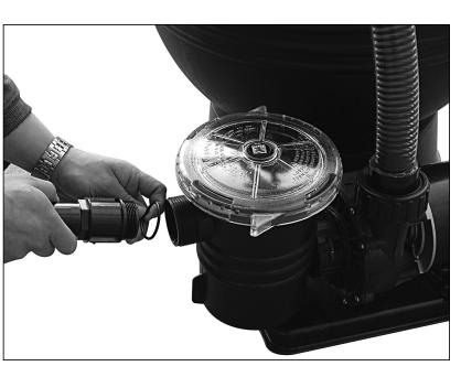
12. Put O-ring over thread on 1½" smooth straight hose adapter and thread into front of pump basket.
