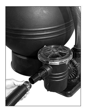
14. Install 6 ft. corrugated hoses by loosening hose clamps and sliding over hose ends. Install hose onto pump basket hose fitting by pushing on and tightening clamp. Install other end of hose onto skimmer and tighten clamp.
