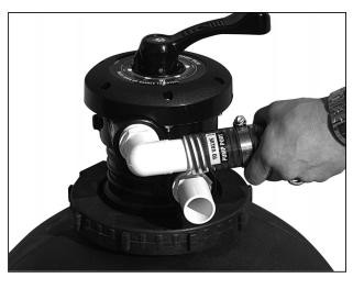
10. Install pump hose labeled "TO VALVE PUMP PORT" by sliding hose with metal clamp over smooth 90° adapter and tighten clamp.
