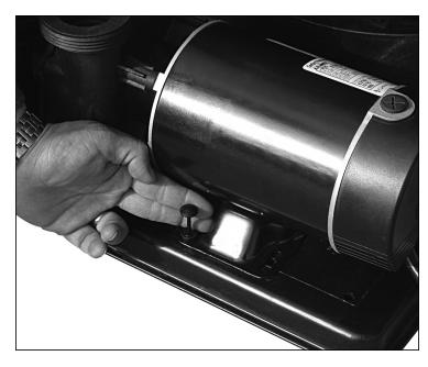
8. Install anchors into slots of pump into holes in pump base. Push pins into anchors to secure.
