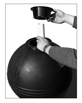
2. Turn filter over. Place next to pool 3. By using a Phillips screwbetween skimmer and return opening on pool. Place sand filter guide in filter over stand pipe. Add approximately 3 inches of water before adding sand. Add required #20 grade silica sand: See sand chart on back page. Remove sand fill guide and save.
